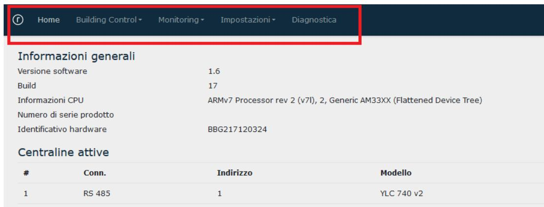
The screenshot shows the YHC web interface. At the top, there is a dark blue navigation bar with a home icon and the following menu items: Home, Building Control (with a dropdown arrow), Monitoring (with a dropdown arrow), Impostazioni (with a dropdown arrow), and Diagnostica. Below the navigation bar, the main content area is titled "Informazioni generali" and displays the following information:
